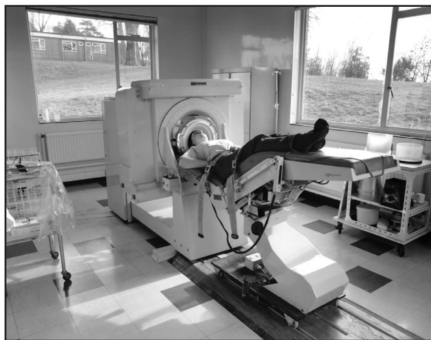
Figure 4. One of the world's first clinically used CT machines, installed in Atkinson Morley Hospital, Wimbledon, England, 1971. (Public Domain)
