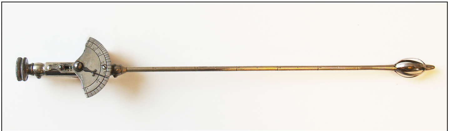
Figure 5. "Urethra-meter," more commonly known as a urethrometer, developed by Fessenden Nott Otis (1825-1900), to measure the appropriate caliber of the sounding tool required for urethral dilation. (Courtesy, WP Ddidusch Museum, Linthicum, Maryland)
